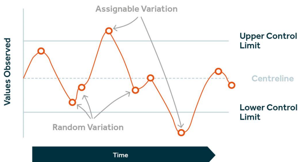
Figure 3: SPC chart – The further a data point is from the centreline the more chance that there is an identifiable cause for the variation and the opportunity to intervene. These assignable variations therefore facilitate targeted interventions.
